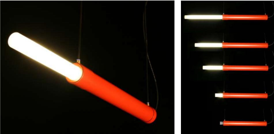
These lights work in the same way as a pneumatic cylinder. The luminous part moves in and outwards by using air pressure. This way you can control the light intensity, and use the lamp both as mood light as well as a work light.
